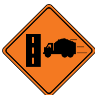
Truck entrance left/right The location at which trucks are entering, leaving or crossing
