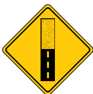
Pavement ends Continuation has gravel surface
