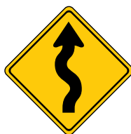
Winding road ahead First curve right
