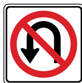
No U-turn You must not turn your vehicle around in the roadway to travel in the opposite direction
